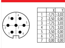
Contact arrangement (Plug-in side)
